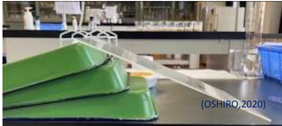
PICTURE: Customized viscosity measuring device.
